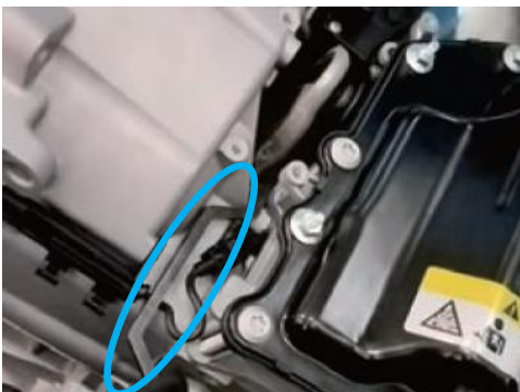
④ After installing the snap ring, use a special tool to turn the fork 2-3 times to eliminate the gap between the snap ring and the clutch.
