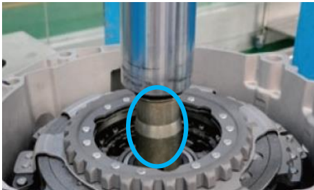
② Stand the gearbox vertically, install the selected washers on the release bearing first, then install the clutch vertically. Use the special indenter with the pressing tool to press the clutch into place. Note: Hammer is strictly prohibited.
