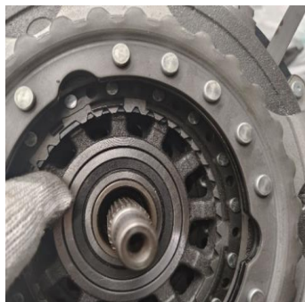
⑤ Use feeler gauges to measure the clearance of the K1/K2 clutch in three measuring points. K1/K2 clearance must be between 0.5-0.8mm at all measuring points.
